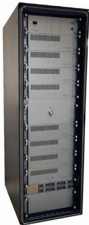
AM96 -1.35-20K 1.3GHz 20kW pulsed 10% duty with 8 power modules
