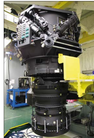
Hyper Suprime-Cam. The instrument weighs 3 tonnes and is 3 m high. (Credit: NAOJ.)
